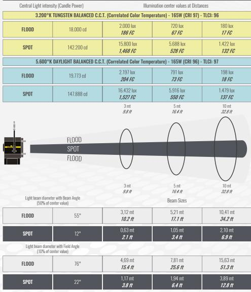
LUX AT ANY DISTANCE = Candle Power: [Distance(in m.)]<sup>2</sup>
